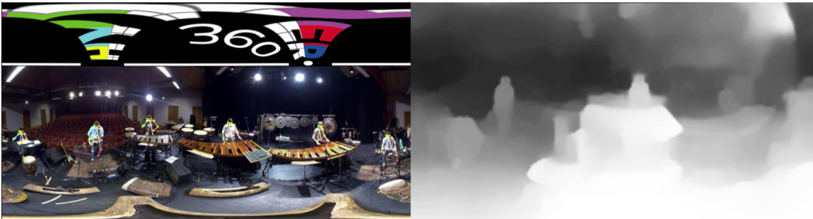
Figure 2: Examples of Artificial Intelligence processing (Left: pose tracking, Right: Spherical depth estimation)
