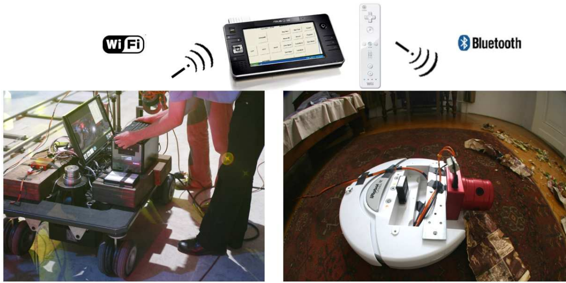
Figure 6: Remote controlled robot camera used to record the panoramic videos for the Metamorphosis (see text for details)
