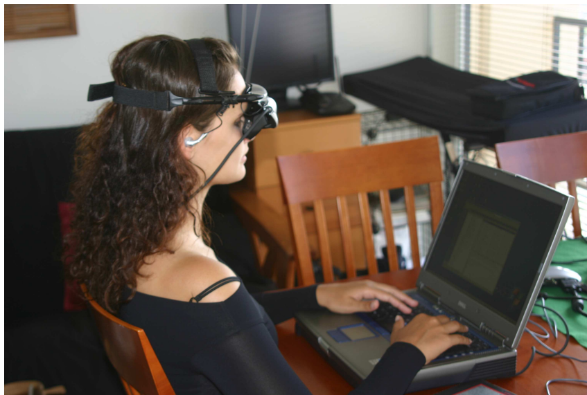
Figure 4: User experiencing full VR immersive interactive reality programming over the Internet using our PanoCAST player, VHIDeviceManager, and built in Physics Engine implemented in Adobe Flash. A range of additional motion sensitive devices, such as a Wii controller or even iPhone/iPad may also be used to control the view point and click on elements in an IP-TV setting.
